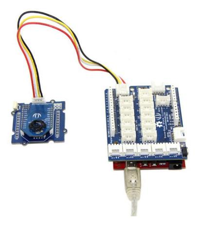
Now you can send some simple AT commands to do some basic configuration for the RF Bee and send/receive data. Of course, you can update the firmware without changing the hardware connection.
