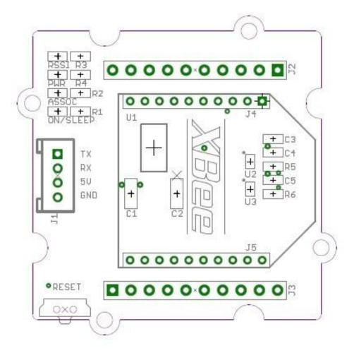
**J1:** Grove Interface, used for connecting to UART Interface of Arduino/Seeeduino.
