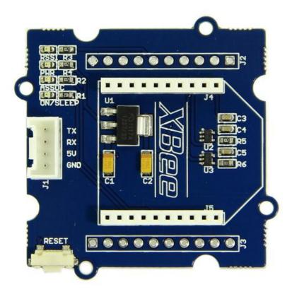
Grove - Bee Socket is an adapter of Xbee serials which can connect wireless modules with Arduino, such as WIFI Bee, RF Bee, Bluetooth Bee, etc. It is Arduino compatible and more effective to conduct operations of peer to peer and mesh network ran by wireless modules. Regulator CJT1117 guarantees Xbee of stable 3.3 voltage. LEDs can perform work modes of the grove clearly. Grove-
