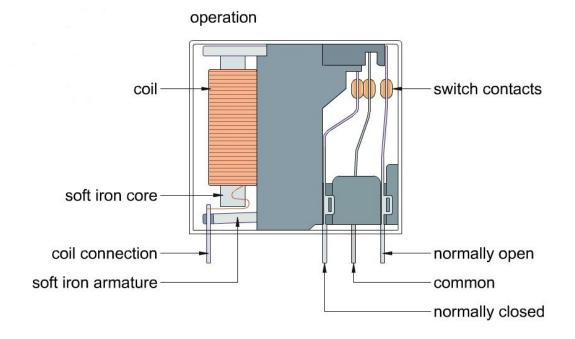
You may see that the common terminal and the normally closed terminal have continuity When the coil of the relay is at rest.
