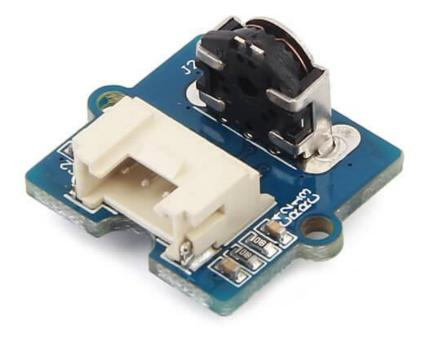
Grove - Mouse Encoder is a type of mechanical incremental rotary encoder with feedback data of rotary direction and rotary speed<sup>[1]</sup>. It features standard Grove interface that will save your lots of work in wiring and programming. Also, it is well adapted to heavy duty and a harsh environment. This product can be applied in toys, robots, and consumer input devices.
