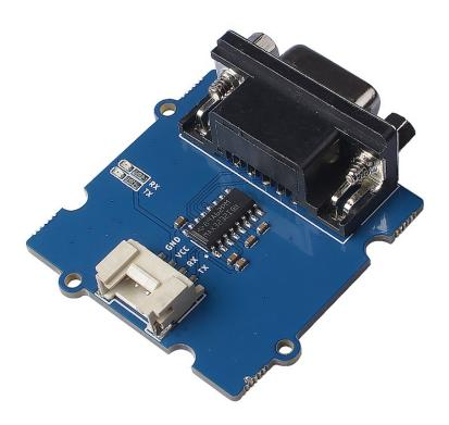
Most of the MCUs use TTL levels, and the computer serial port generally uses 232 levels. If we want the computer to communicate with the MCU, we need this **Grove - 232**. Communication between your Arduino and your computer will be exceptionally convenient with the integrated Grove interface
