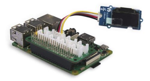
Tap the following command <code>grove\_oled\_display\_128x64</code> in the command line interface.
