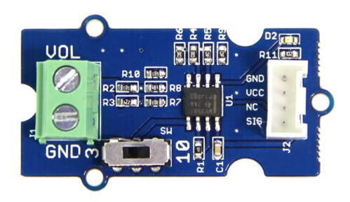
The Grove – Voltage Divider provides an interface for measuring external voltage, eliminating the need to connect a resistance to input interface. Besides, the voltage gain can select by dial switch. They are easy to use.
