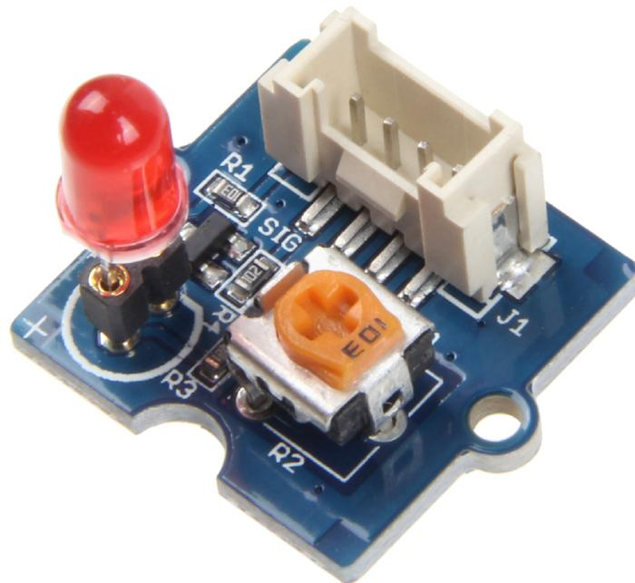
Grove - Red LED is similar to the Grove - LED module which houses an LED light source. In addition, it also has a potentiometer on-board to manage the power requirements of the LED. The PCB of this module has mounting holes which can be mounted on the required surface of your prototype. For example, it can be used as a pilot lamp for indicating power or signal presence.
