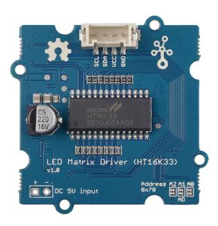
LED Matrix is low cost and usually used to display simple numbers and images. The Grove - LED Matrix Driver is the I<sup>2</sup>C based product which allows you to control the LED matrix with our prepared and easy-to-use libraries, or you can create your own library to control it to satisfy your need. The 8\*8 LED Matrix can be assembled and unassembled from the driver board easily, so it is convenient to change different color LED matrix display based on your need.
