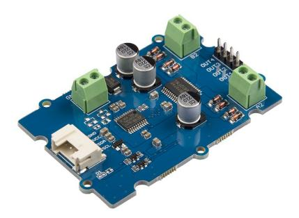
The Grove - I2C Motor Driver (TB6612FNG) can drive two DC motors up to 12V/1.2A or drive one stepper motor up to 12V/1.2A. With the on-board MCU, it can work with Arduino easily via the Grove I2C interface. This diver board is based on TB6612FNG, which is a driver IC for DC motor and stepper motor with output transistor in LD MOS structure with low ON-resistor. Two input signals, IN1 and IN2, can choose one of four modes such as CW, CCW, short brake, and stop mode.
