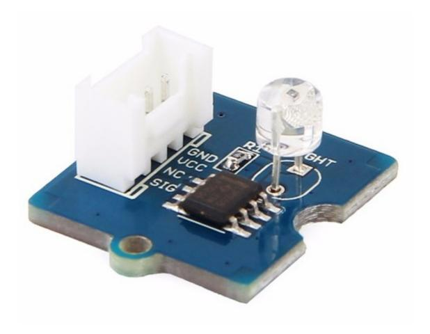
The Grove - Light sensor integrates a photo-resistor(light dependent resistor) to detect the intensity of light. The resistance of photo-resistor decreases when the intensity of light increases. A dual OpAmp chip LM358 on board produces voltage corresponding to intensity of light(i.e. based on resistance value). The output signal is analog value, the brighter the light is, the larger the value.
