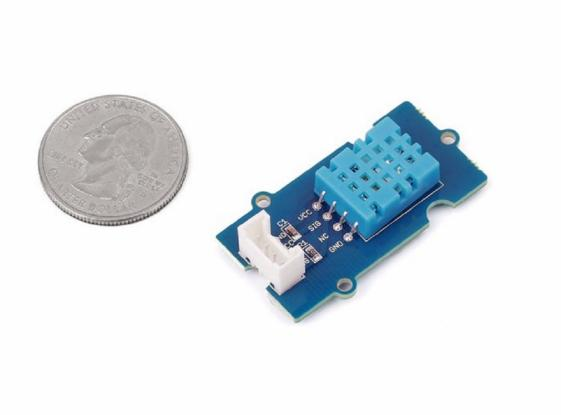
This temperature & humidity sensor provides a pre-calibrated digital output. A unique capacitive sensor element measures relative humidity and the temperature is measured by a negative temperature coefficient (NTC) thermistor. It has excellent reliability and long term stability. Please note that this sensor will not work for temperatures below 0 degree.
