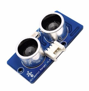
This Grove - Ultrasonic ranger is a non-contact distance measurement module which works at 40KHz. When we provide a pulse trigger signal with more than 10uS through singal pin, the Grove\_Ultrasonic\_Ranger will issue 8 cycles of 40kHz cycle level and detect the echo. The pulse width of the echo signal is proportional to the measured distance. Here is the formula: Distance = echo signal high time \* Sound speed (340M/S)/2. Grove\_Ultrasonic\_Ranger's trig and echo singal share 1 SIG pin.
