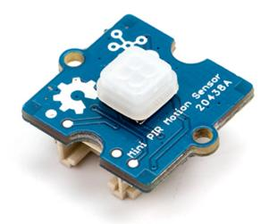
Grove - mini PIR motion sensorallows you to sense motion, usually human movement in its range. Simply connect it to Grove - Base shield and program it, when anyone moves in its detecting range, the sensor will output HIGH on its SIG pin.
