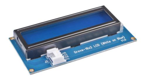
This Grove – 162 LCD module is a 16 Characters 2 Lines LCD display, it uses I2C bus interface to communicate with the development board, thus these will reduce the pin header from 10 to 2 which is very convenient for the Grove system. This LCD display module also supports customise characters, you can create and display heart symbol or stick-man on this LCD module through a simple coding configuration.
