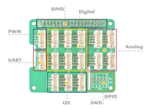
GPIO: The same pin out as the raspberry pi.
