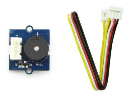
This module uses piezo buzzer as the main component, it can produce high pitch tone while it is connected to digital output and logic level set to High, otherwise it can produce various tones according to the frequencies generated from the Analog PWM output that connected to it. (note: the frequency range that normal human ear can distinguish is between 20 Hz and 20kHz.)
