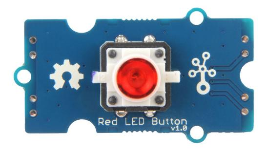
The Grove - LED Button is composed of Grove - Yellow Button, Grove - Blue LED Button and Grove - Red LED Button. This button is stable and reliable with a 100 000 times long life. With the build-in LED, you can apply it to many interesting projects, it is really useful to use the LED to show the status of the button.
