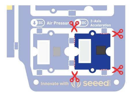
Looking closely at the Grove Beginner Kit For Arduino you will see that there are 3 small holes between each individual module and the backplane. All you need to do is cut the PCB backplane around the module from the small holes using a pair of diagonal pliers.
