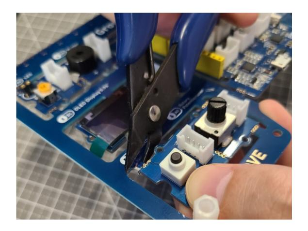
Note: carefully cut along the periphery of the small hole, do not cut to the small hole (to prevent internal wiring short circuit and thus damage the module); if you accidentally cut to the small hole, please use a knife to clean the small hole to prevent short circuit
