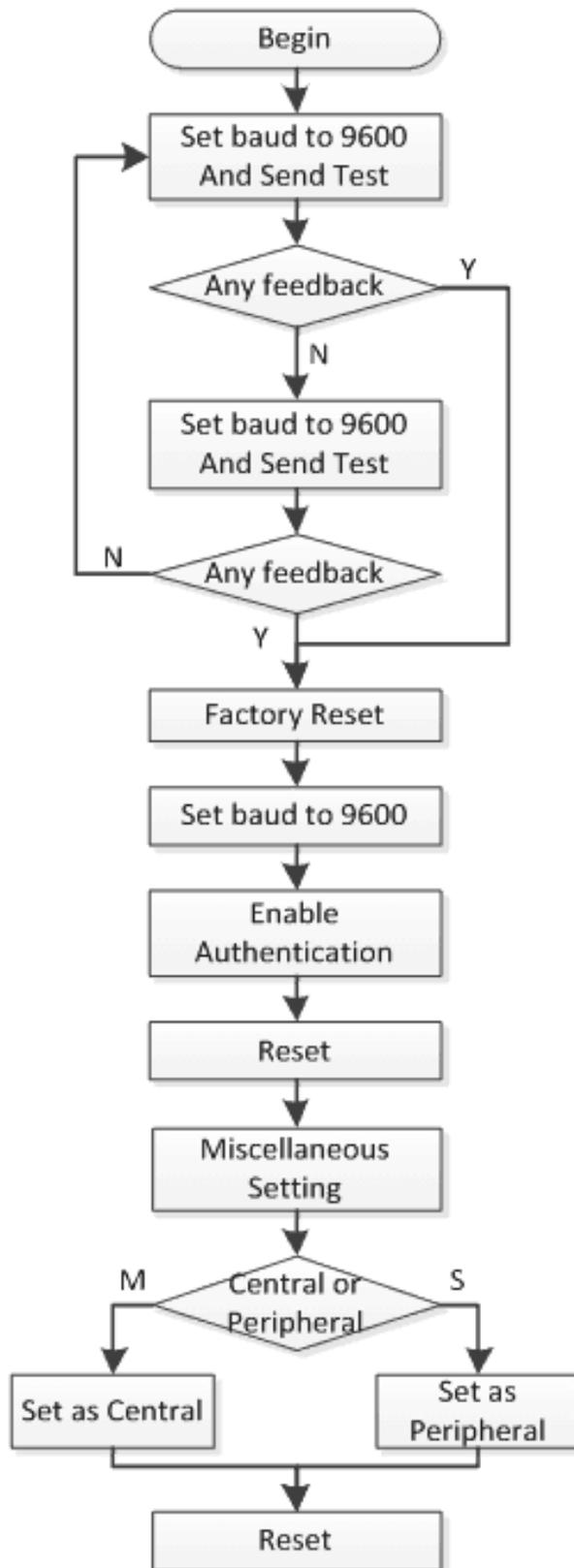
After the initialisation, the Central and Peripheral will do different things, the Central will send message to Peripheral interval and print
