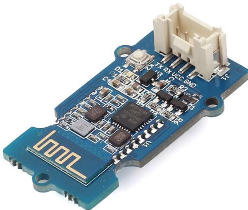
Grove - BLE (dual model) v1.0 uses CSR dual mode Bluetooth chip. The chip is based on ARM architecture and supports AT instructions. Users can develop flexibly according to the serial baud rate, equipment name, pairing password.
