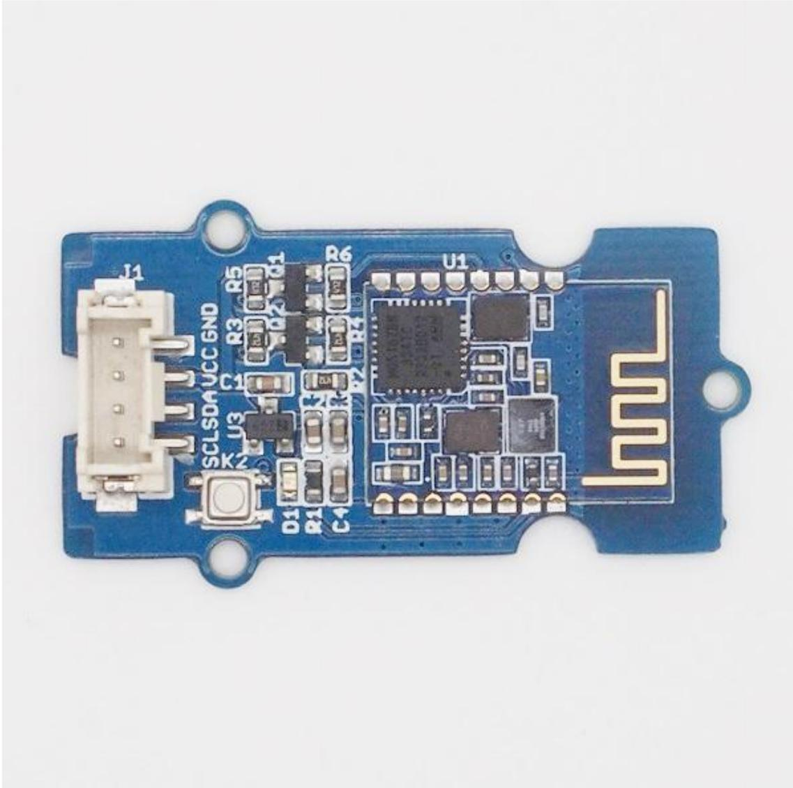
**K2:** During connected status, it could be disconnected by pressing K2 button more than 100ms. During sleep mode, it could be restored through pressing K2 (factory settings) button.
