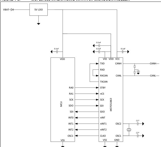
FIGURE 1-3: MCP251863 INTERFACING WITH A 5V MICROCONTROLLER
