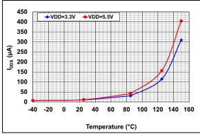
**FIGURE 10-1:** Average IDDS vs. Temperature.
