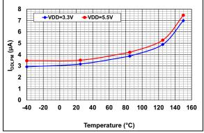
**FIGURE 10-2:** Average IDDLPM vs. Temperature.
