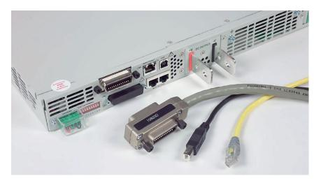
Figure 2. Built-in Ethernet, USB 2.0, and GPIB interfaces enable easy system connections.
