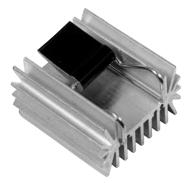
Ohmite's R2 Series (patent pending) heatsink provides a large surface area along with our C Series clipping mechanism to attach to a TO-247 or TO-264 package. The self-aligning features of the clip assure secure attachment and enhanced thermal performance. Because no screws are required for device mounting, additional fins can be added to the rear side of the heatsink for increased total surface area in a more compact space.
