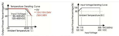
Note: 1. With an AC input voltage between 85-115VAC and a DC input between 120-163VDC the output power must be derated as per the temperature derating curves;
