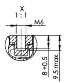
In case of no tolerance shown in dimensional drawing, general tolerances apply: dimension  $\leq$  10 mm;  $\pm$  0.3 mm; dimension 10 to 50 mm;  $\pm$  0.6 mm; dimension > 50 mm;  $\pm$  1 mm
