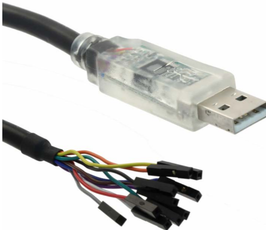
Figure 8. FTDI USB to I2C Dongle
