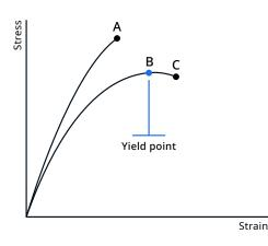
A. Tensile stress at break, elongation at break (no yield point)B. Tensile stress at yield, elongation at yieldC. Tensile stress at break, elongation at break
