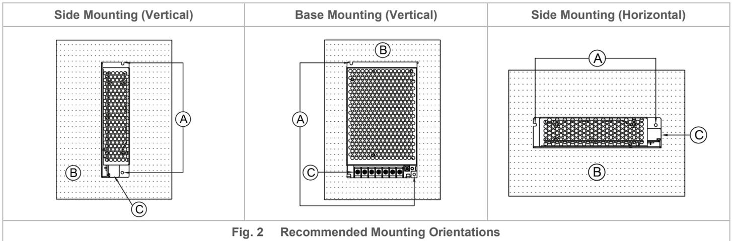
Fig. 2 Recommended Mounting Orientations
