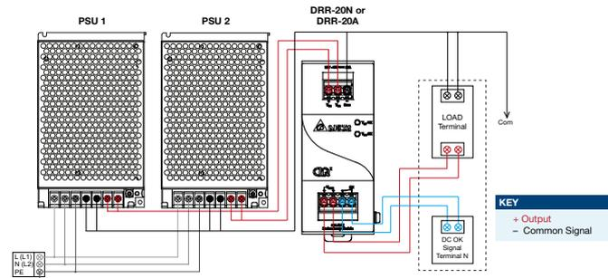
Fig. 5 Redundancy Operation Connection Diagram
