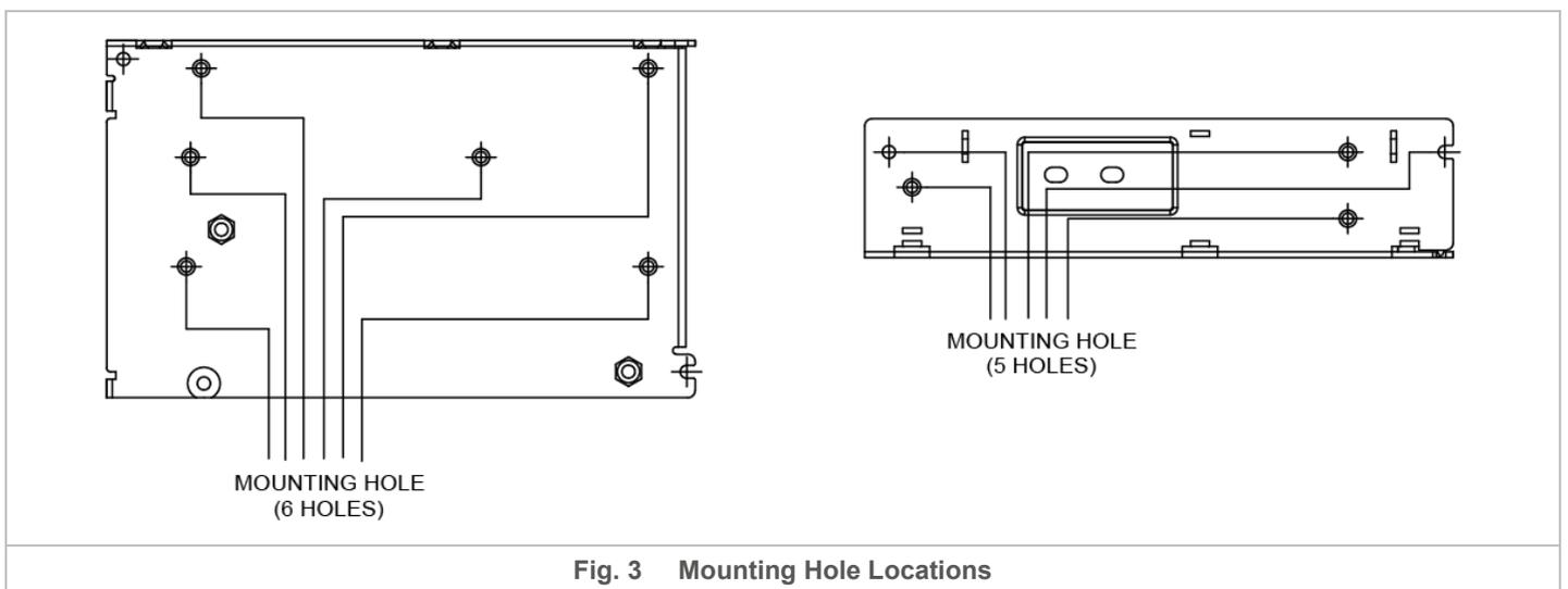
Fig. 3 Mounting Hole Locations
