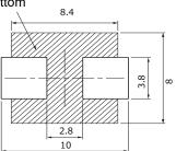
③Parts arranged around this power choke coil do not touch the surface of this power choke coil (Top side and side). (Series MC)
