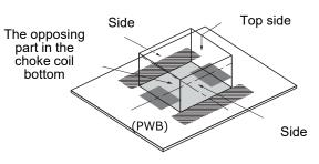
④This power choke coil is different from the ferrite core-type that installs general concentration GAP. It has the leakage magnetic bunch distribution of the choke coil to the vertical direction. Please be cautious when using parts and circuit compositions which are easily affected by the leakage flux.
