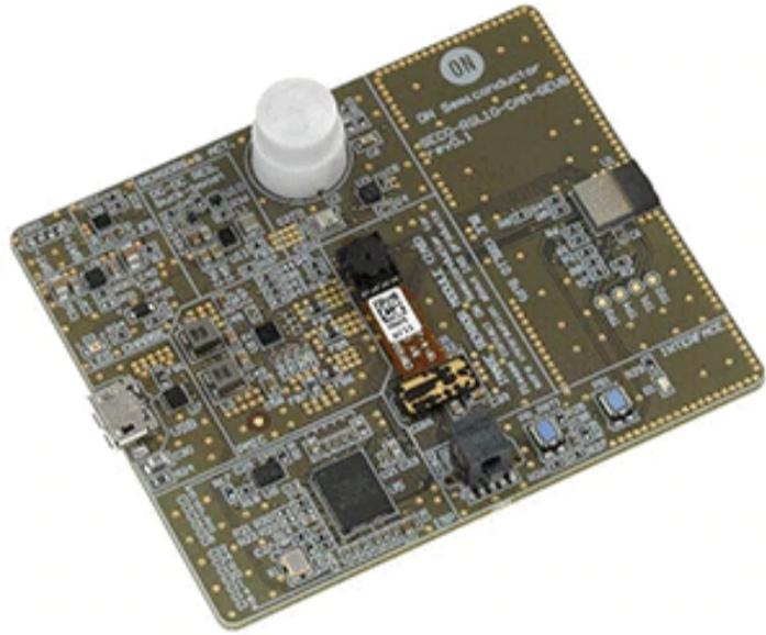
The RSL10 SIP serves as the processing hub of the camera, enabling Bluetooth® Low Energy connectivity of captured image and sensor data to the provided mobile app (available on [GooglePlay™](#), [iOS®](#)).
