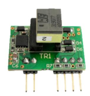
regulator, enabling a low component count, compact and robust design. Among the features of this converter stand out – e.g. an internal temperature compensated reference, a controlled duty cycle oscillator with an active current limit circuit, driver and high current output switch. The board is realized with Automotive qualified parts and is pin compatible with commercial IGBT DC/DC supplies, provisioning a ready to use plug–in solutions for power applications.
