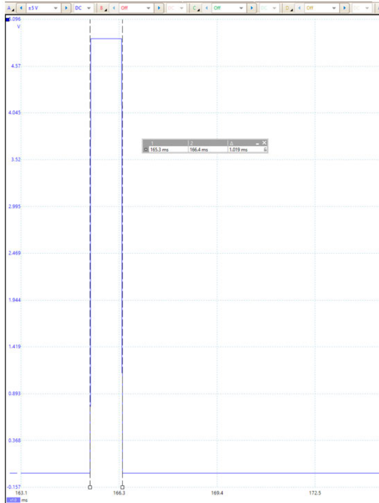
Figure 15. Enable pulse signal waveform generated by an external MCU connected to the AEK-POW-LDOV01J
