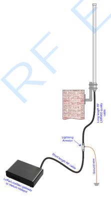
This setup where gateway is far from the antenna requires longer outdoor cable. Typically the RF cable length outdoors being more than 2-3 meters is considered enough to configure the way depicted in the figure.
