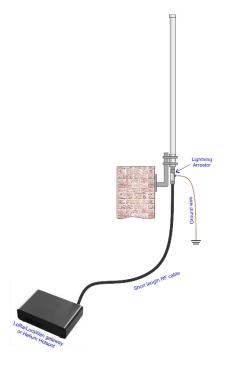
This is the simplest case and best option if the gateway is not far from the antenna, typically the RF cable length outdoors should be 2 meters or less, although cable length indoors may be larger.
