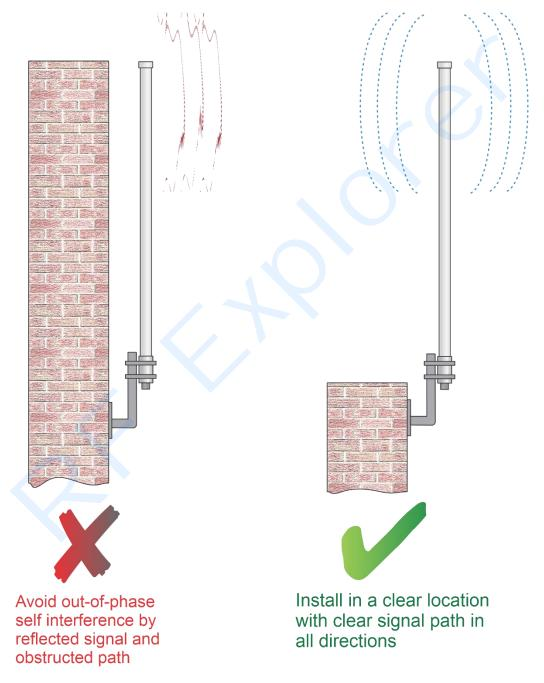
2) If the antenna is installed on a location with metallic objects nearby, make sure the antenna is always above such objects and as far as possible. Metallic objects and surfaces negatively impact in antenna VSWR and signal reflections.
