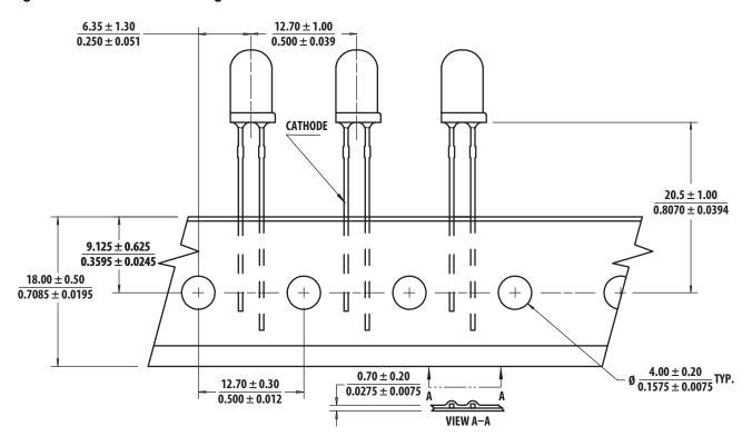
**NOTE:** The ammo-packs drawing is applicable for packaging option –DD and -ZZ and regardless standoff or non-standoff.
