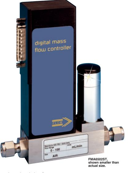
tube are heated, and when flow takes place, gas carries heat from the upstream to the downstream windings. The resultant temperature differential is proportional to the change in resistance of the sensor windings.
