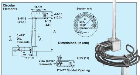
tank. These heaters are convenient answers for many immersion. Heating applications capacities, dimensions and sheaths fit a wide range of heating applications. Easy to install and remove for cleaning with straight or circular element designs to fit many tank configurations.
