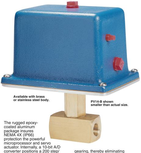
revolution stepper motor for precise flow. The stepper motor is directly connected to the valve stem without backlash (hysteresis) effects. The valve can also be manually controlled with a screwdriver.
