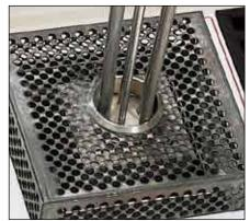
CL950 multi-well accepts up to 5 probes at one time and comes standard with %, %, % and two %" diameter holes.
