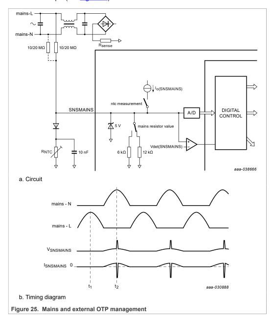
The TEA6017AT continuously measures the SNSMAINS voltage via an A/D converter and waits until it detects a peak (t1). This peak value is internally stored and used for the mains compensation. The output of the A/D converter is used for brownout/brownin detection.
