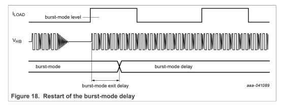
When the LLC is switching for a time that exceeds the burst-mode exit delay time and the output load exceeds the burst-mode level, the system leaves the burst mode. The burst-mode delay function is activated again. The burst-mode exit delay time can be set with a parameter.
