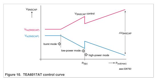
When the output power ( $P_{out}$ ) is at its maximum, the low capacitor voltage level ( $V_{ls(SNSCAP)}$ ) is at its minimum and the high capacitor voltage ( $V_{hs(SNSCAP)}$ ) is at its maximum level. The maximum  $\Delta V_{SNSCAP}$  ( $V_{hs(SNSCAP)} - V_{ls(SNSCAP)}$ ), which is the divided  $\Delta V_{Cr}$  voltage, corresponds to the maximum output power.
