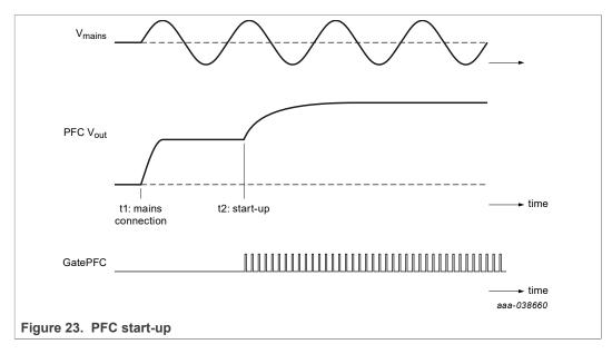
At t1, the mains is connected and the PFC output voltage equals the peak voltage of the mains. At t2, the PFC starts switching and its output voltage increase in line with an RC curve.
