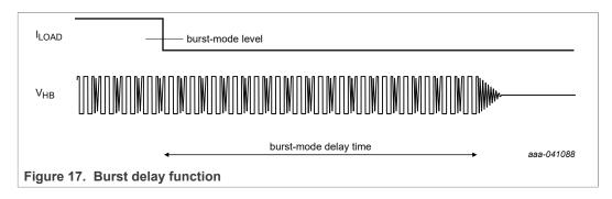
If, during the burst-mode delay time, the output voltage cannot be regulated properly and continues to increase, the system enters burst mode anyway.
