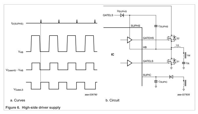
The external bootstrap buffer capacitor  $C_{SUPHS}$  supplies the high-side driver. The bootstrap capacitor is connected to the low-side driver supply, the GATELS pin, and the half-bridge node (HB) via an external diode ( $D_{SUPHS}$ ). When GATELS is active high and the HB node is pulled low,  $C_{SUPHS}$  is charged.
