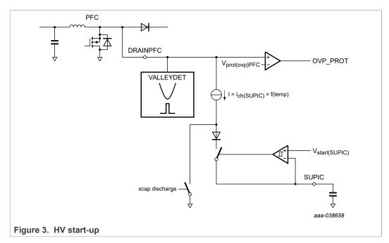
The maximum current of the internal current source is limited to  $I_{ch(SUPIC)}$ . To limit the IC dissipation, the charge current is reduced when the current source exceeds its maximum temperature.
