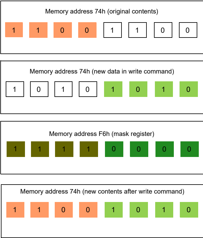
Figure 145. Example of I 2 C Byte Write Bit Masking
