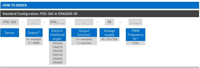
1 The analog output is ratiometric, proportional to input voltage
