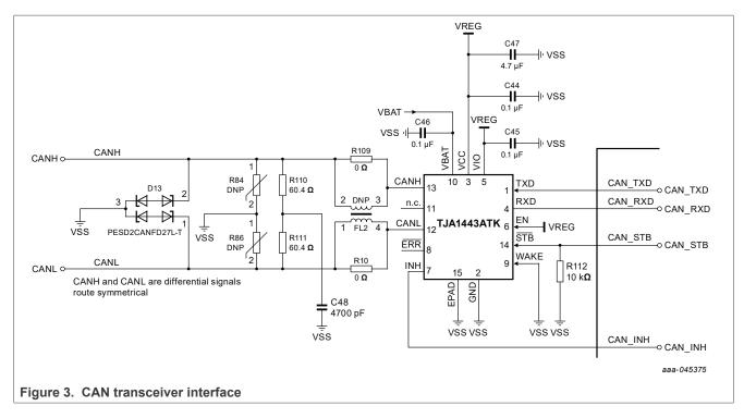
Check the need of external 120  $\Omega$  termination when interfacing CAN tools to RD33775ACNCEVB. If necessary, populate R84 and R86 with 60  $\Omega$  resistors.
