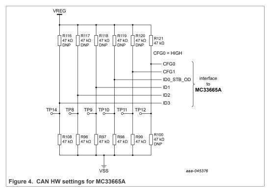
Based on the circuit shown in <u>Figure 4</u>, CFG0 is set to HIGH and CFG1 is set to LOW. CAN communication can be established with 500 kbit/s of baud rate and CAN FD arbitration baud rate is fixed at 500 kbit/s. ID0\_STB\_OD, ID1, ID2, and ID3 are set to zero.
