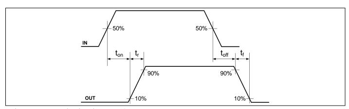
Figure 6 Switching time waveforms
