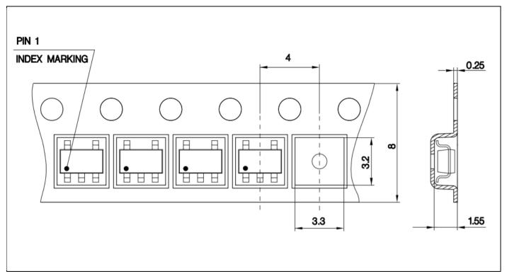
Figure 14 Tape and reel dimensions
