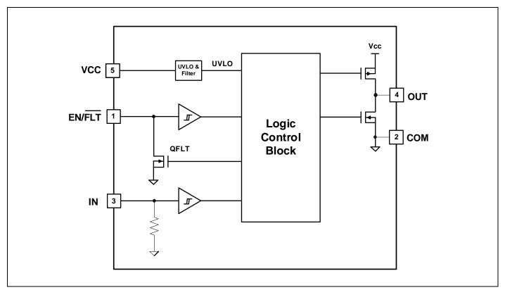
Figure 2 Block diagram
