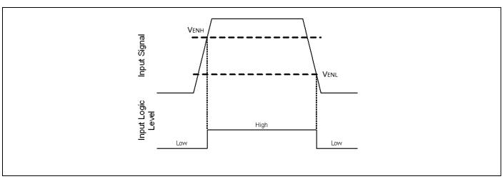
Figure 12 EN input thresholds
