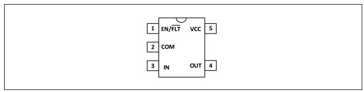
Figure 3 PG-SOT23-5-1 (top view)
