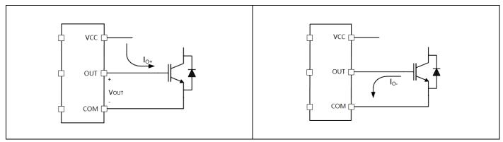
Figure 4 Gate output sourcing current
