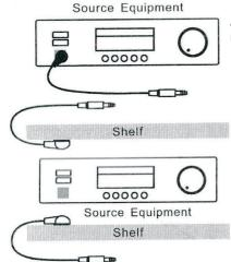
Attached directly to the equipment - most reliable method.
