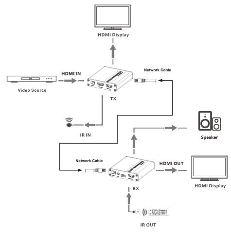
One to one connection with IR remote up to 70 metres over HQ CAT6 cable.
