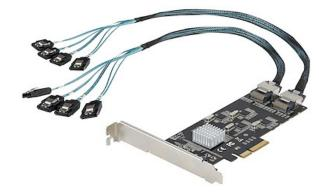
This 8-port SATA III (6Gbps) controller enables you to add eight SATA 6Gbps hard drives (HDDs) or solid State Drives (SSDs) to your computer system or server via an available PCIe x4 card slot. The card supports SATA III and PCI-Express Gen 2 Specifications and four SATA controllers to deliver a high-performance data storage solution.
