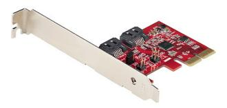
This 2-port SATA III (6Gbps) controller with RAID enables you to add two SATA 6Gbps Hard Drives (HDDs) or Solid State Drives (SSDs) to your computer system or server via an available PCIe x2 card slot, and build the disks into a hardware RAID array. The card supports SATA III and PCI-Express 2.0 Specifications, and can also be used to add optical disk drives (ODD) like CD/DVD/Blu-ray to your computer.
