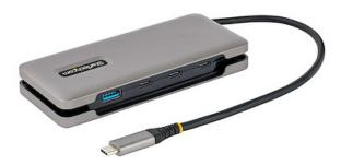
This 4-Port USB-C Hub expands the connectivity of a USB-C laptop. This hub features four USB 3.2 Gen 2 (10Gbps) enabled ports, three USB-C and one USB-A, that support high-bandwidth USB peripherals. Connect the attached USB-C cable to a USB Type-C or Thunderbolt 3/4 port, located on the host computer, to enable the quick connection of up to 4 peripherals.
