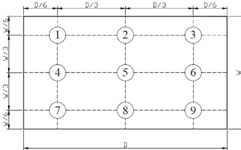
$$B\text{-uni} = (\text{Minimum luminance of 9 points} \div \text{Maximum luminance of 9 points}) \times 100\%$$
