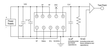
Figure 8. Phase Noise Clipped Sine Test Circuit (No I<sup>2</sup>C Control)
