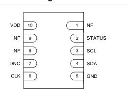
Figure 2. Pin Assignments (Bottom view)
