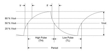
Figure 10. Clipped Sinewave Waveform Diagram<sup>[13]</sup>
