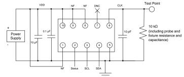
Figure 6. LVCMOS Test Circuit (I<sup>2</sup>C Control)
