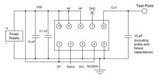
Figure 4. LVCMOS Test Circuit (No I<sup>2</sup>C Control)
