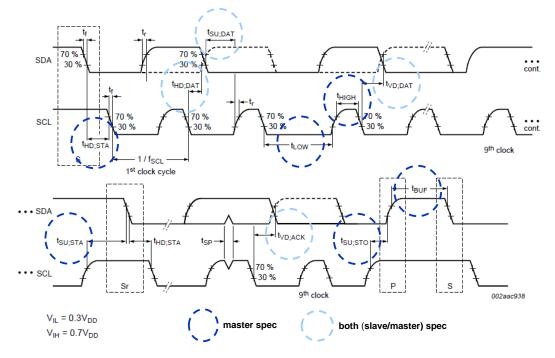
Figure 24. I<sup>2</sup>C Timing Diagram
