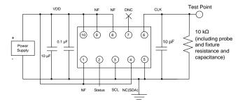
Figure 5. Clipped Sinewave Test Circuit (No I<sup>2</sup>C Control)
