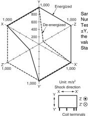
Sample: G6DN-1A Number of Relays: 5 pcs Test conditions: Impose a shock in the ±X, ±Y, and ±Z directions three times each with the Relay energized to check the shock values that cause the Relay to malfunction. Standard:100 m/s²
