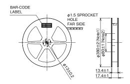
Note1:The (53) specification is  $\phi$ 180 $\pm$ 2. Note2:The (53) specification is  $\phi$ 60 $\pm$ 1.
