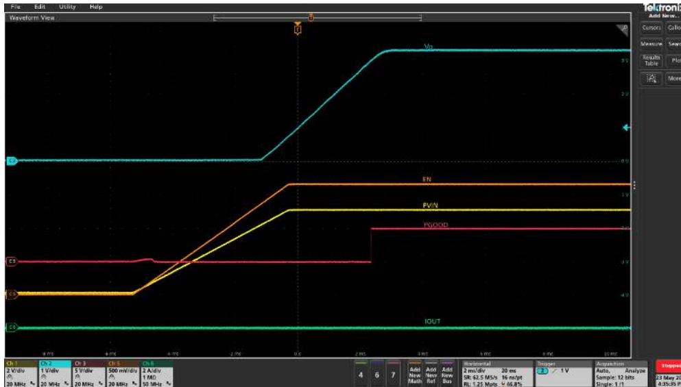
Figure 13 Startup with no load (Ch1:PV IN , Ch2: V OUT , Ch3: PG, Ch5: Enable, Ch8:I OUT )
