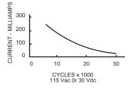
One cycle is  $360^{\circ}$  rotation clockwise and  $360^{\circ}$  return. The data for the curve was measured at sea level,  $25^{\circ}$ C and 68% relative humidity with the life limiting criteria which follows.
