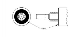
Panel is sealed by a flat rubber seal washer at the base of bushing. Shaft is sealed by an O-ring inside the bushing. After the switch is mounted, seals do not alter the dimensions of the unsealed style.
