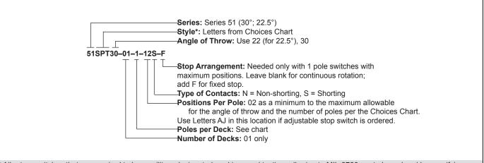
\* All rotary switches that are required to have military designated markings and testing adhering to MIL-3786 are to be ordered by specifying the military part number identified on the appropriate slash sheet.
