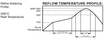
WAVE SOLDERING: 260°C maximum solder temperature for 5 seconds max. \*\* Note: 100% matte tin terminal plating does not meet MIL-S-83504 for lead content.
