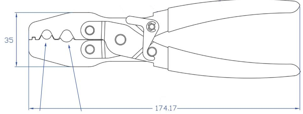
O.D. Max: 6.0mm O.D. Max: 8.5mm
